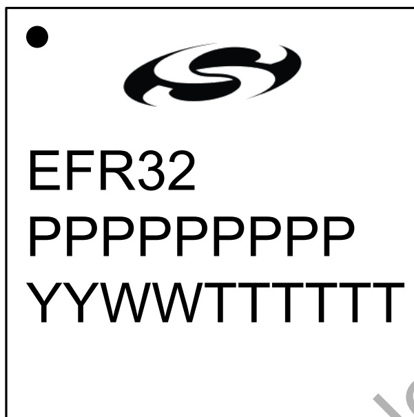
Figure 8.3. QFN32 Package Marking
