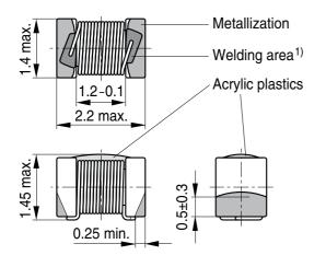
1) This area (30% of contact area) should not be used to assess solderability
