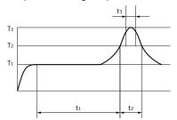
$T1 = 150 \text{ to } 180^{\circ}\text{C}$  $T2 = 230^{\circ}C$
