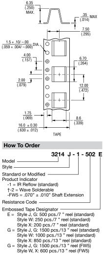
Consult factory for other available options. + -2 has a treated stainless steel shaft Tape and reel material meets Antistatic ANSI/ ESD 5541-2003 packaging standards.
