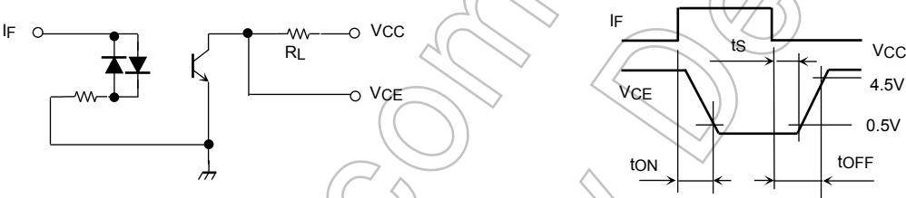
Fig. 1: Switching operating conditions
