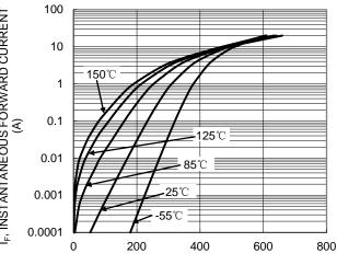
$V_{\text{F}}$ , INSTANTANEOUS FORWARD VOLTAGE (mV) Figure 2. Typical Forward Characteristics
