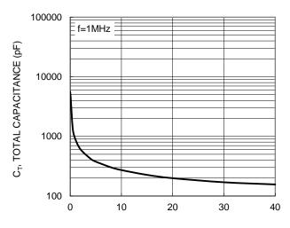
$\rm V_R$ , DC REVERSE VOLTAGE (V) Figure 5. Total Capacitance vs. Reverse Voltage
