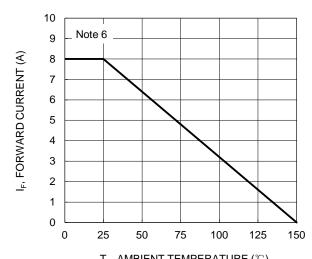
$T_A$ , AMBIENT TEMPERATURE (°C) Figure 4. Forward Current Derating Curve
