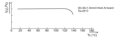
T.S.D is capable of starting operation at Tc 120 to 130 $^{\circ}$ C. When this is converted to junction temperature (Tj) according to the formula below.
