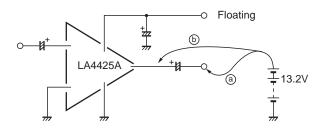
The power pin is in a floating state when a power capacitor is connected, so if  $+V_{CC}$  touches output lines (a) and (b), the upper power transistor inside the IC will be damaged.
