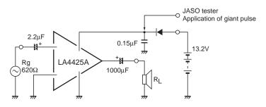
The over-voltage protector (V<sub>CC</sub>X  $\approx$  21.5V) inside the IC is used to cut all bias routes and reverse bias between B-E of output stage elements, in order to increase the power line's capability of handling positive surge. This means, of course, that a V<sub>CES</sub> (V<sub>CBO</sub>) type output stage element is used instead of the V<sub>CEO</sub> (V<sub>CER</sub>) type.
