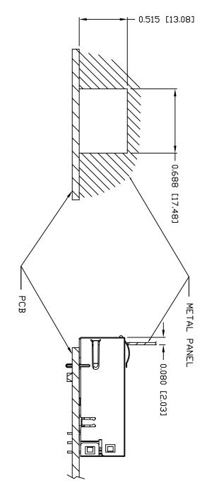
IN CASE THIS DISTANCE IS DIFFERENT, THE REQUIRED PANEL OPENING DIMENSIONS CHANGE ACCORDINGLY. THE DISTANCE OF PANEL INSIDE SURFACE RELATIVE TO FRONT SURFACE OF PART IS ONLY A SUGGESTION
