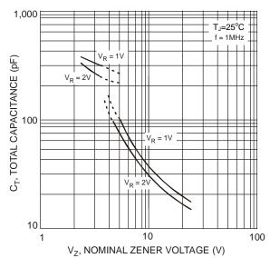
Fig. 4 Typical Total Capacitance vs. Nominal Zener Voltage
