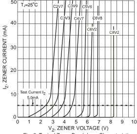
Fig. 2 Typical Zener Breakdown Characteristics
