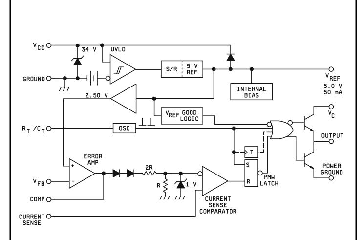
NOTE: Toggle flip flop used only in device types 03, 04, 07, and 08.
