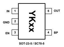
NOTE1: The location of pin 1 on the YKxx is determined by orienting the package marking as shown.
