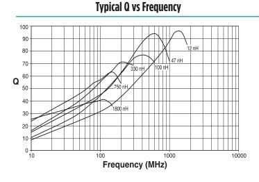
2. Q measured using a HP4291A RF Impedance Analyzer with a HP16193A Test Fixture
