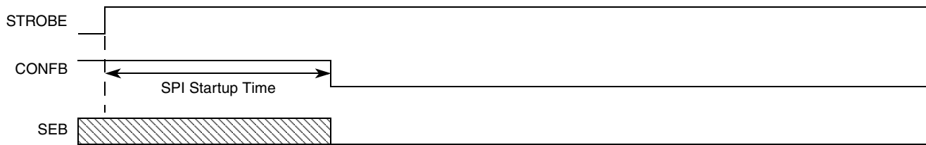
Figure 21. Valid Sequence from Standby/LVD Mode to Configuration Mode
