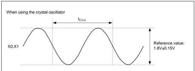
The amplitude changes by resistance, capacity which added outside or the difference of the device.
