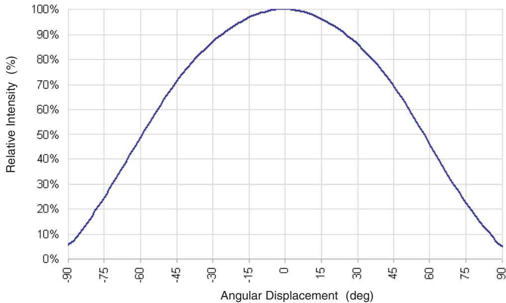
Figure 1 Ia. Typical representative spatial radiation pattern for cool-white and neutral-white lambertian.
