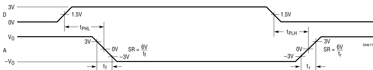
Figure 15. V.28 Driver Propagation Delays
