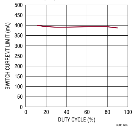
Switch Current Limit vs Duty Cycle
