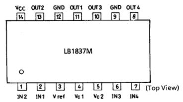
Note: Both GND pins must be grounded.
