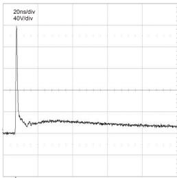
Figure 6 ESD Response to IEC 6100-4-2 (+8kV Contact Discharge)
