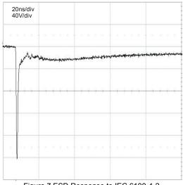
Figure 7 ESD Response to IEC 6100-4-2 (-8kV Contact Discharge)
