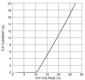
Figure 8 Transmission Line Pulsing (TLP) Current vs. Voltage
