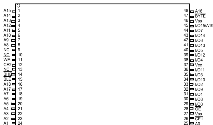
Figure 3. 48-pin TSOP I pinout (Top View) [1, 3]
