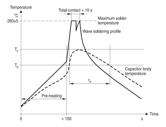
T<sub>s</sub>: Capacitor body maximum temperature at wave soldering
