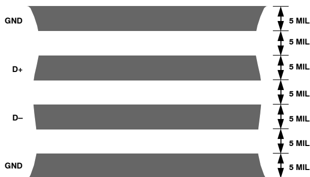
Figure 22. Typical Arrangement of Signal Tracks
