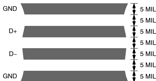
Figure 21. Typical Arrangement of Signal Tracks
