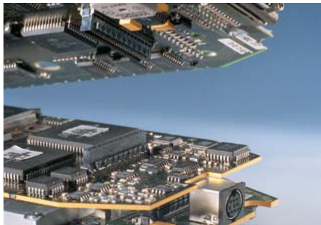
Mezzanine cards in mobile phone test equipment
