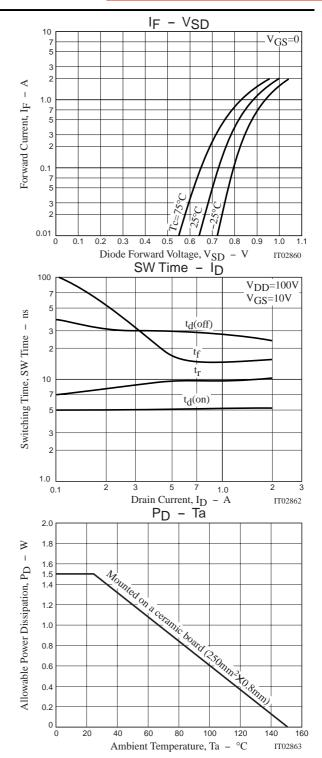
Note on usage : Since the 2SK2951 is designed for high-speed switching applications, please avoid using this device in the vicinity of highly charged objects.
