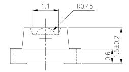
For reflow soldering (propose)
