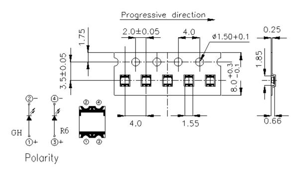
Note: The tolerances unless mentioned is  $\pm 0.1$ mm ,Unit = mm
