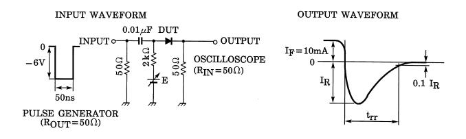
Fig.1 Reverse recovery time (trr) test circuit
