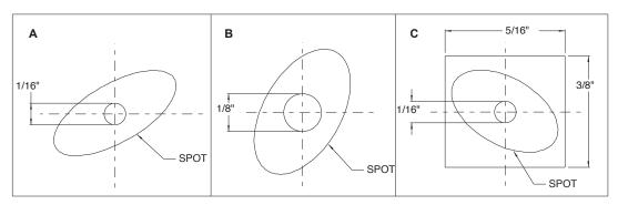
A. 750 footcandles minimum over a B. 750 footcandles minimum over C. 750 footcandles minimum over a 1/16" DIA. circle centered on the axis of the lamp.
