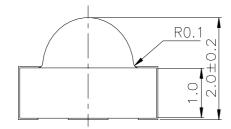
For reflow soldering (propose)
