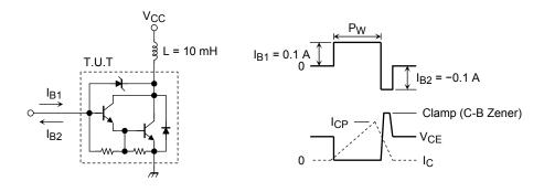
Note 2: (1) Pulse width adjusted for desired  $I_{CP}$  ( $I_{CP}$  = 5.47 A min)
