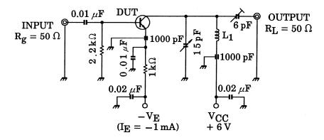
$L_1$ : 0.8 mm $_{\phi}$  silver plated copper wire, 4 T, 10 mm ID, 8 mm length
