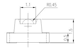
For reflow soldering (propose)
