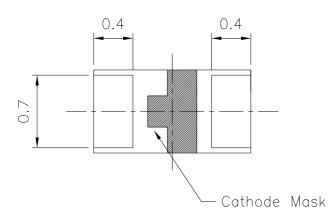
For reflow soldering (propose)
