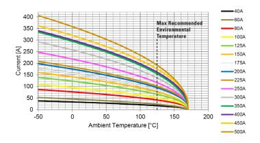
Derating curves may change depending on the final condition of the application (terminals characteristics, wire
