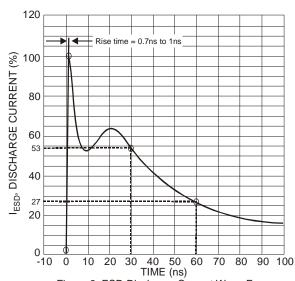
Figure 2 ESD Discharge Current Wave Form IEC 61000-4-2 (330Ω/150pF)
