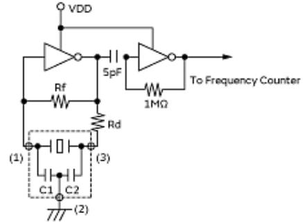
Regarding CERALOCK<sup>®</sup> with built-in capacitors, the terminal (1) and (3) are interchangeable, but if connection is interchanged, the specification of initial tolerance frequency may not be guaranteed.
