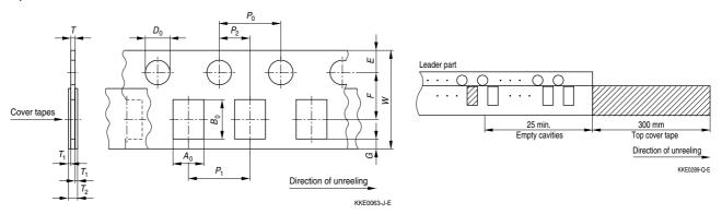
Dimensions and tolerances in mm for case size 0402:
