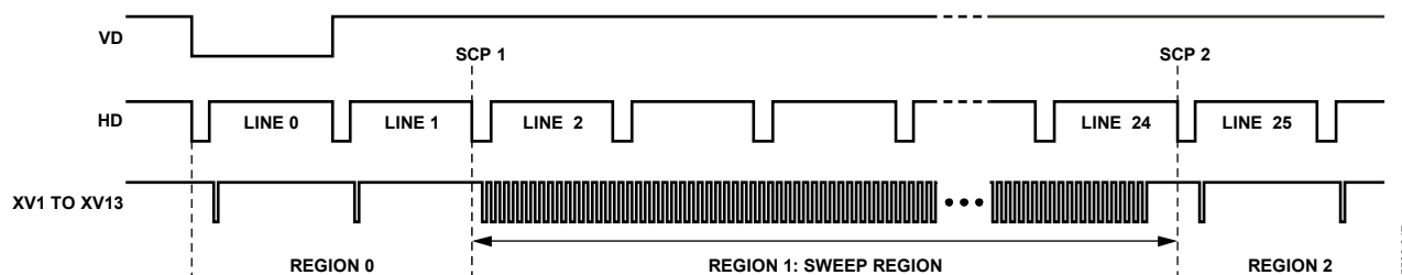
Figure 48. Example of Sweep Region for High Speed Vertical Shift
