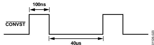
Figure 21. \overline{\text{CONVST}} When Temperature Channel Selected
