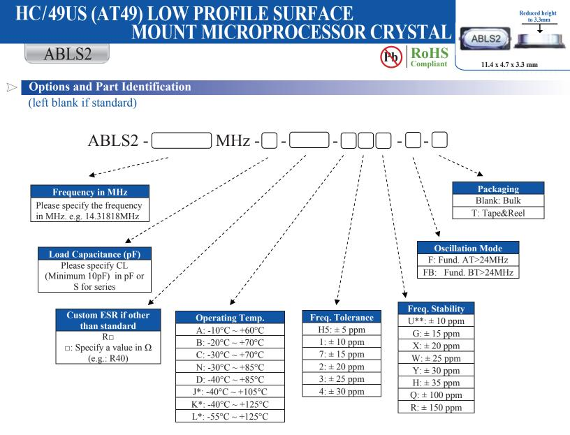
NOTE: Fundamental BT frequency stability  $\pm$  100ppm max. at -10° C to +60° C only.
