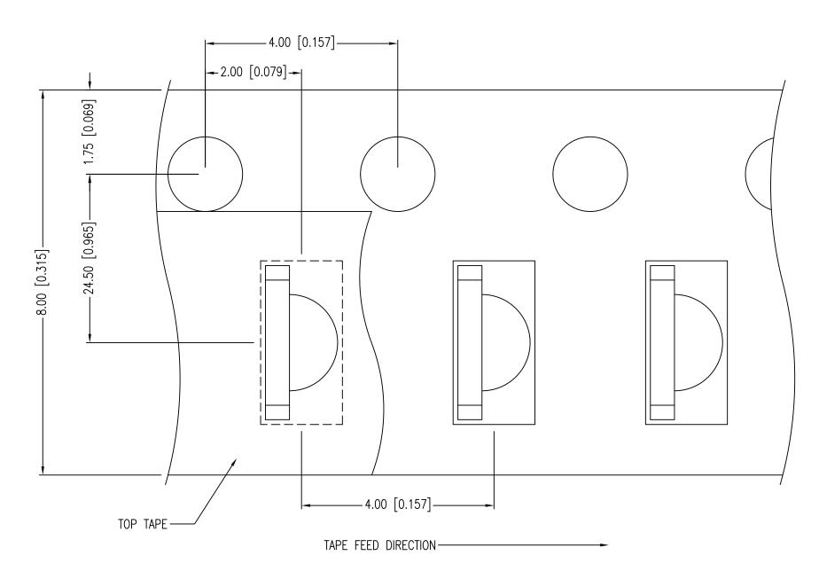
\*UNLESS OTHERWISE SPECIFIED TOLERANCES PER DECIMAL PRECISION ARE: X= $\pm 1$  ( $\pm 0.039$ ), X.X= $\pm 0.127$  ( $\pm 0.002$ ), LEAD SIZE= $\pm 0.05$  ( $\pm 0.002$ ), LEAD LENGTH= $\pm 0.75$  ( $\pm 0.030$ ). MIN=  $^{+DECIMAL}_{-0.00}$  PRECISION MAX.=  $^{+0.00}_{-0.00}$  MAX UNCONTROLLED DOCUMENT
