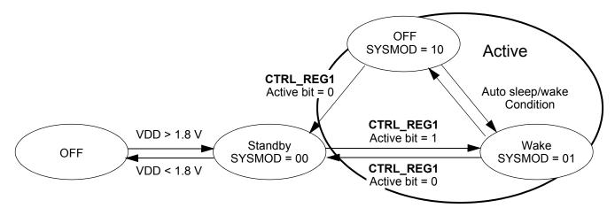
Figure 6. Mode transition diagram
