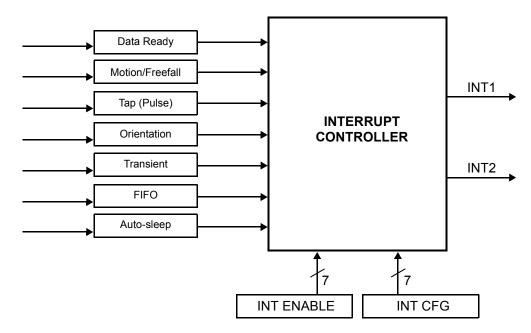
Figure 10. System interrupt generation block diagram
