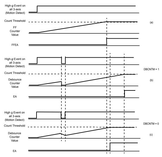
Figure 13. DBCNTM Bit Function
