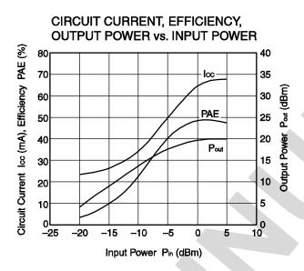
Condition: f = 2 450 MHz, Vcc1 = Vcc2 = Vbias + Venable = 3.0 V, Pin = 0 dBm, with external input and output matching circuit
