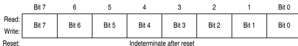
Figure 14-13. TIM Channel Register Low (TCHxL)
