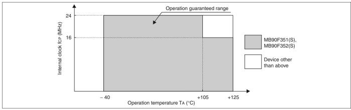
WARNING: The recommended operating conditions are required in order to ensure the normal operation of the semiconductor device. All of the device's electrical characteristics are warranted when the device is operated within these ranges.
