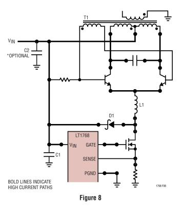
together with minimum trace between them. If space constraints prohibit the transformer T1 placement next to C1, local bypassing (C2) for the center tap of transformer T1 should be used.
