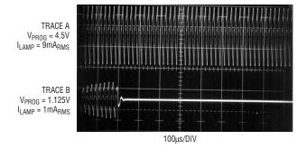
Figure 3b. CCFL Current for Circuit in Figure 1
