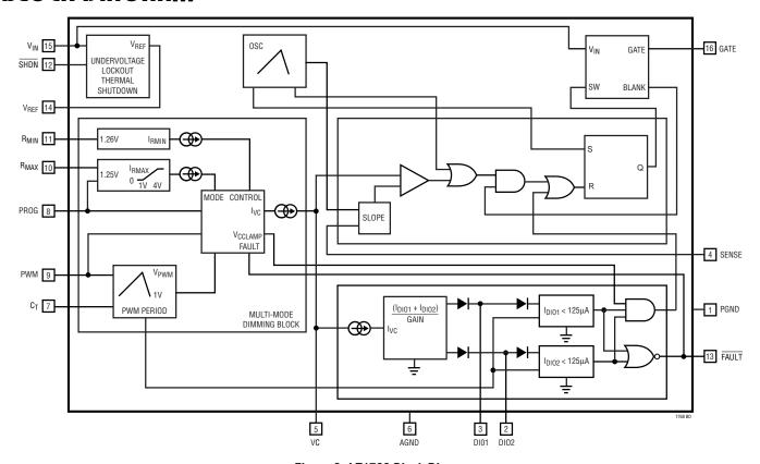
Figure 2. LT1768 Block Diagram
