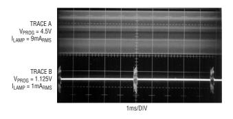
Figure 3a. CCFL Current for Circuit in Figure 1
