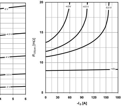
8 Typ. drain-source on-state resistance
