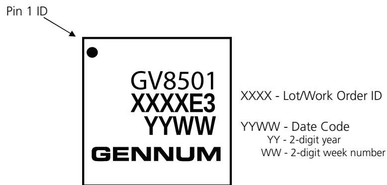
Figure 6-3: GV8501 Marking Diagram
