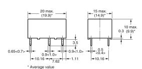
Dimensions in pointed brackets < > are for the Relay mounted to Socket(-P6C).
