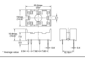
PCB Mounting Holes (BOTTOM VIEW) Tolerance: ±0.1 mm
